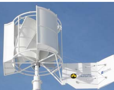
IAMU's logo is proudly displayed on the turbine's rudder, which helps steer the unit into the wind at the proper angle.
